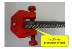
One bolt is retracted too much. Make it protrude 3 mm or more before tightening.
