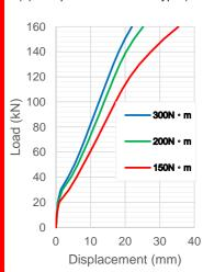
As a result of changing the tightening torque value and checking the performance of the product using steel material having a mill scale surface as shown in the graph on the left, there was almost no difference between the specified torque values of 300 N · m and 200 N · m, but the displacement increased with 150 N · m. Therefore, we have set the initial torque to 300 N · m in order to always apply 200 N · m.
